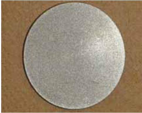
Figure 6. Sintered stainless steel filter.
