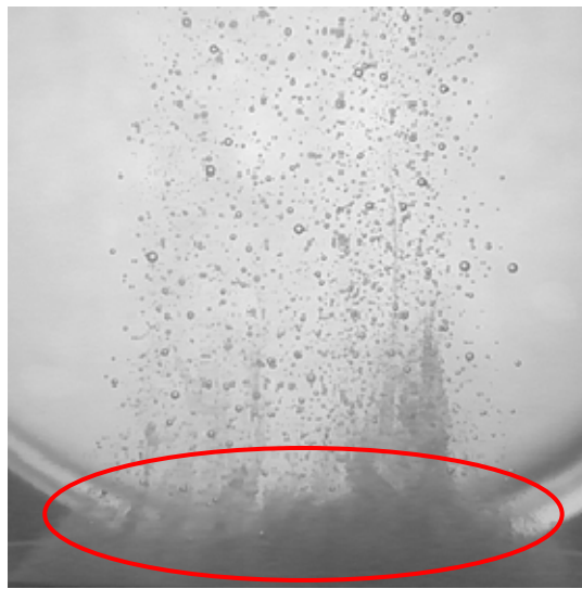
Figure 10. Behavior of injected CO 2 microbubbles (40°C, 10 MPa)
